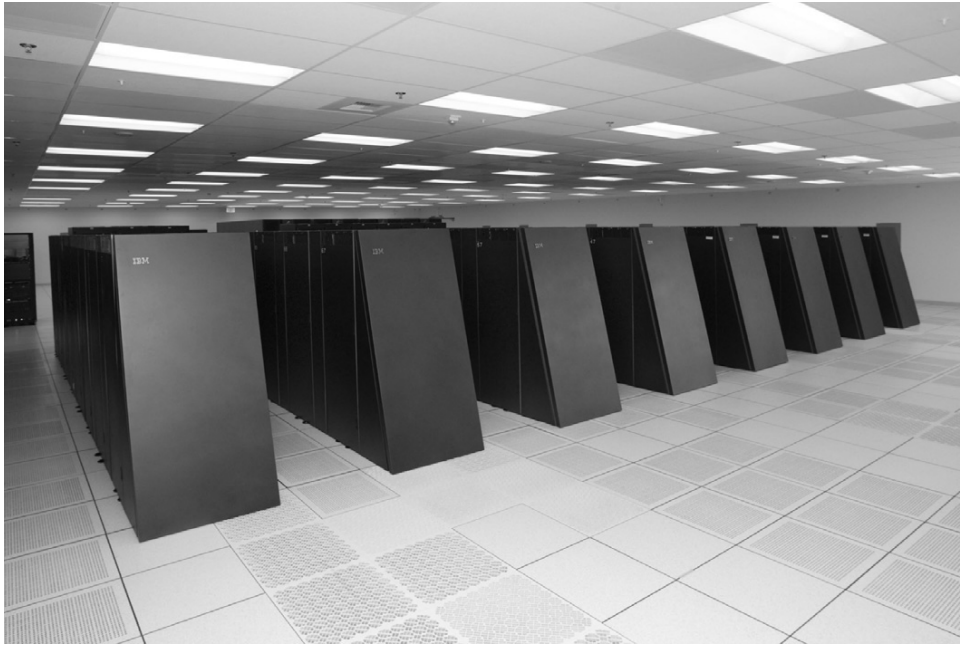
Figure I.19 The 64K-processor Blue Gene/L system.
