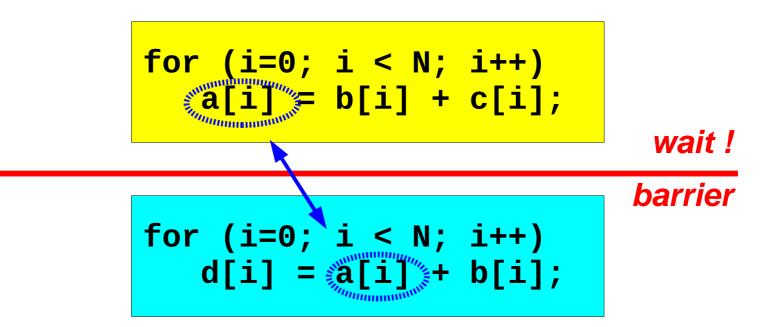
All threads wait at the barrier point and only continue when all threads have reached the barrier point
